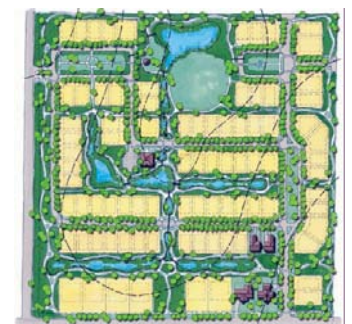
In a conventional subdivision layout, the entire site is converted to roads and building lots (above). Below is the same area with the same number of building lots using low-impact design. (Conservation Design Forum 2003)
