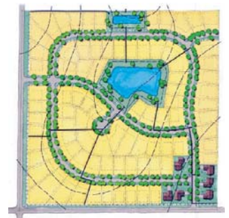
In a conventional subdivision layout, the entire site is converted to roads and building lots (above). Below is the same area with the same number of building lots using low-impact design. (Conservation Design Forum 2003)
