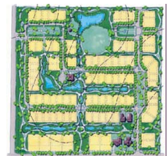
In a conventional subdivision layout, the entire site is converted to roads and building lots (above). Below is the same area with the same number of building lots using low-impact design. (Conservation Design Forum 2003)
